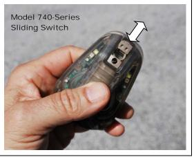
Main Switch: 0=Off, Functions 1 & 2 Nose SW/Plug: ▲=Mode A, ▼=Mode B
